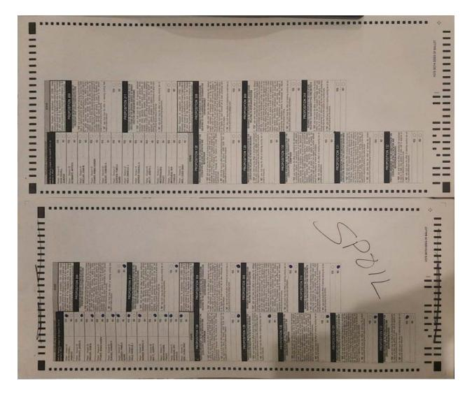
11. The large black rectangles at three of the four corners enable detection of which end of the ballot is the top, since ballots may be inserted into the tabulator in either direction.
